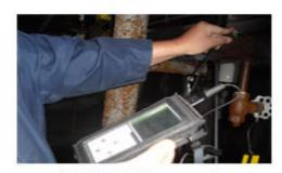
NDT Ultrasonic Thickness Measurements
